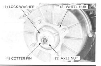
Remove the drum cover mounting bolts.
