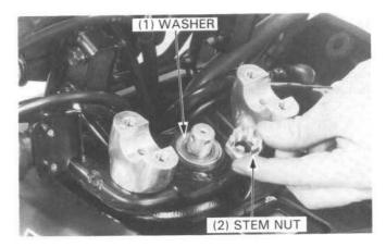
Tighten the steering stem nut to 80 N·m (8.0 kg-m, 58 ft-lb) torque first. Then tighten the nut further to align the hole of the shaft with the groove of the nut.
