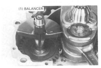
Disassemble the transmission (page 10-7). Remove the crankshaft from the left crankcase using a hydraulic press.
