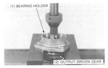
Place the bearing holder in the press and remove the bearing.
