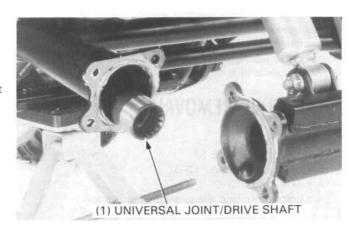
Inspect the universal joint bearings for excessive play or damage.
