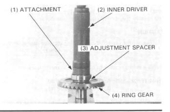
If necessary, drive the ring gear bearing into the cover.
