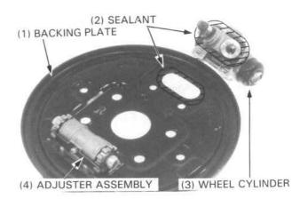
Install the wheel cylinder and adjuster assemblies onto the brake backing plate.
