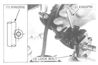
Tighten the kingpin lock nut to the specified torque value.
