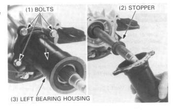
Drive the axle out using a plastic hammer from the left side.
