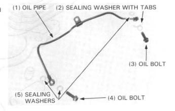
Install the oil pipe with the oil bolts, sealing washers and 6 mm bolt.
