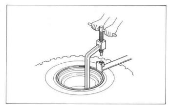
Screw in the breaker arm compressor bolt to break the bead from the tire.
