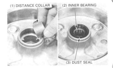
Apply grease to the dust seal lip and install the dust seal and side collar.
