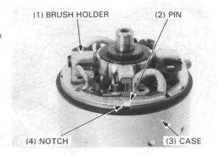
Install the rear cover aligning its slot with the brush holder pin.
