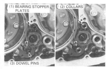
Install the guide plate and drum shifter assembly.
