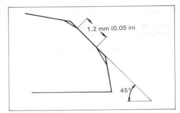
Apply a thin coating of Prussian Blue to the valve seat. Press the valve through the valve guide and onto the seat to make a clear pattern.
