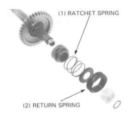
Remove the circlip and disassemble the pinion gear and washers.
