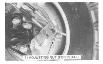
Remove the foot peg/brake pedal mount bolts, cotter pin and washer from the pedal pivot shaft.
