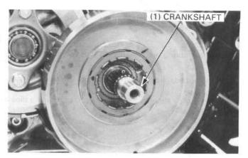
Install the centrifugal clutch weight assembly onto the clutch drum and crankshaft.
