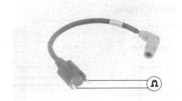
Remove the spark plug cap from the wire and measure the secondary coil resistance.
