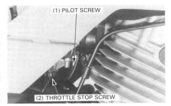
Remove the carburetor (page 4-5) and float chamber.
