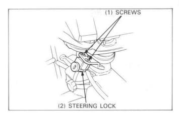
Install the steering lock and tighten the screws. Install the following:
