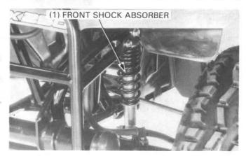
Compress the front shock absorber with the shock compressor, adaptor and atachment.
