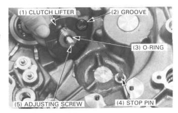
Install the ball retainer onto the clutch lifter.
