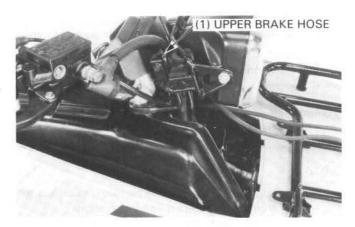
Check the three-way joint and lower hoses for damage and brake fluid leaks.
