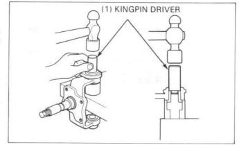
Set the knuckle leg, a new bushing and suitable block, such as a wooden piece, in a vise as shown, and install the bushing in the knuckle leg by tightening the vise.
