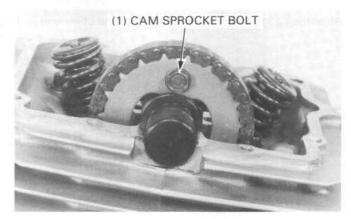
Realign the "T" mark with index mark and recheck the cam sprocket timing marks.
