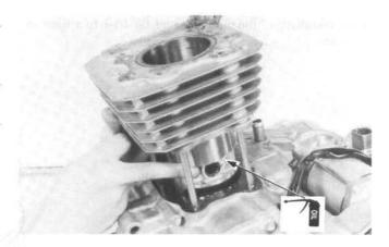
Tighten the cylinder mount bolts.
