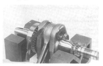
Measure the radial clearance at the connecting rod big end, at two points in the directions indicated by the arrows.
