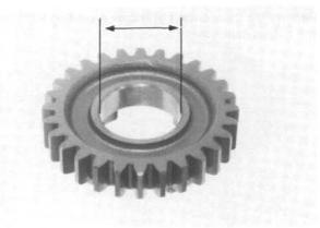
Measure the I.D. and O.D. of each gear bushing.
