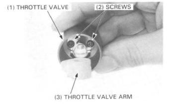
Check the throttle valve and jet needle for wear or damage.
