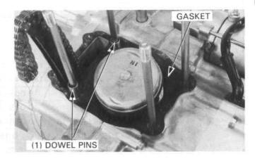
Clean off any gasket material from the cylinder surface.
