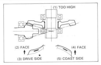
Replace the pinion spacer with a thinner one if the contacts are too low, to the flank side. The patterns will shift about 1.5-2.0~mm (0.06-0.08~in) when the thickness of the spacer is changed by 0.10~mm (0.004~in).
