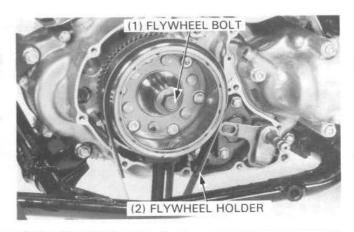
Remove the flywheel with the rotor puller.
