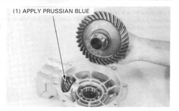
Clean all sealing material off the mating surfaces of the gear case and cover.
