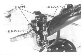
Remove the lower grease nipple from the kingpin.
