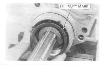
Tighten the drive gear bearing outer race lock nut.
