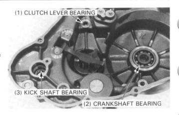
Check the oil seals for wear or damage. Replace them if necessary.
