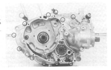
Remove the right crankcase cover bolt. Place the engine with the left crankcase down and remove the right crankcase.
