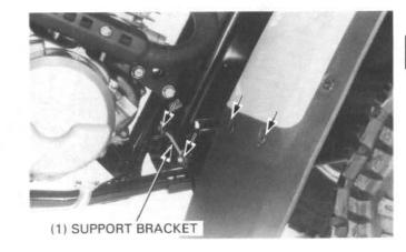
Remove the inner fenders and front fender.
