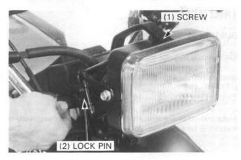
Remove the headlight lower mounting screws and remove the headlight from the headlight case.
