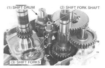
Remove the thrust washer and C1 gear from the countershaft.
