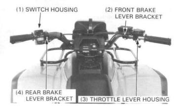
Remove the handlebar upper holder cover cap and cover by removing the bolts.
