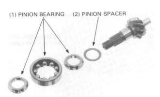
Press the bearing onto the pinion gear shaft with the special tools shown.
