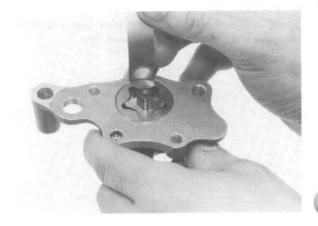
Measure the pump rotor tip clearance.
