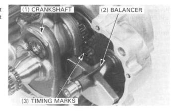
Draw the crankshaft into the left crankcase using the special tools.
