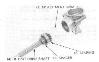
Clean the output gear case in solvent and blow open the oil passage with compressed air.
