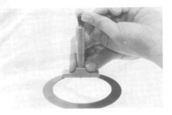
Install the washer and clutch spring.
