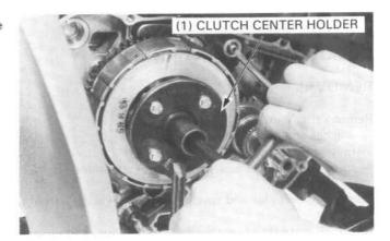
Remove the lock washer, clutch center, discs, plates and pressure plate.
