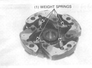
Measure the height of the clutch spring.
