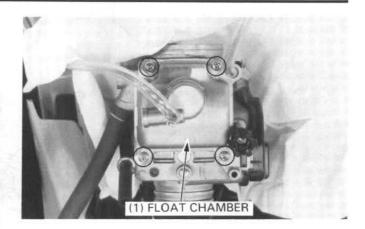
Replace the standard main jet with the high altitude type (#122). Assemble and install the carburetor.
