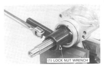
Heat the output gear case around the drive shaft bearing to 80°C (176°F).
