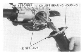
Install the left bearing housing and tighten the bolts.
