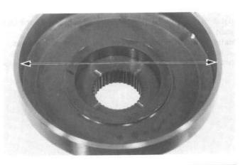
Inspect the one-way clutch for smooth operation and check the rollers for excessive wear.
