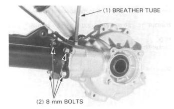
Remove the gear case 10 mm bolts, final gear case, spring and drive shaft from the swing arm.
