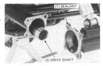
Install the final gear case mount bolts. Tighten the 10 mm bolts first, then the 8 mm bolts.
