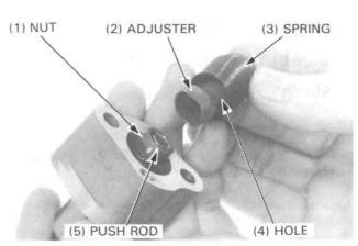
Align the spring hook with the groove in the cover and install.
