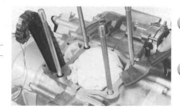
Install the piston and piston pin, using new piston pin clips.
