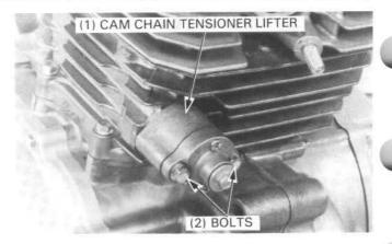
Remove the two screws assembling the cam chain tensioner lifter and disassemble.
