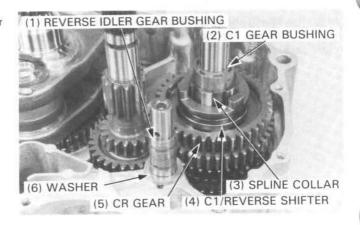
Remove the CR/C2 gear bushing and C2 gear from the countershaft.
