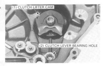
Install the washer, bearing and thrust washer onto the clutch lifter cam.
