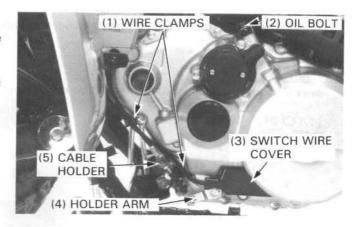
Remove the oil filler cap/dipstick, right crankcase cover bolts and the cover.
