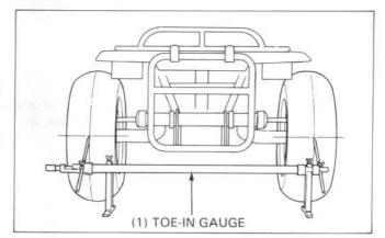
Align the toe-in gauge with the marks on the tires as shown. Check the readings on the gauges scales.
