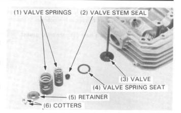
Install the valve spring retainers and install the valve cotters.
