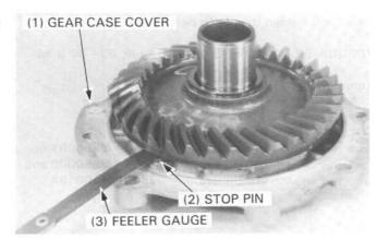
Remove the ring gear. If the clearance exceeds the service limit, heat the gear case cover to approximately 80°C (176°F) and remove the stop pin by tapping the cover.
