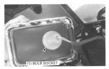
Install a new bulb and the socket.
