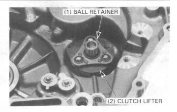
Install the clutch lifter cam by aligning its groove with the clutch lever bearing hole on the right crankcase cover.
