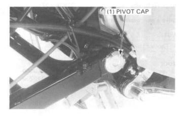
Remove the pivot lock nut.
