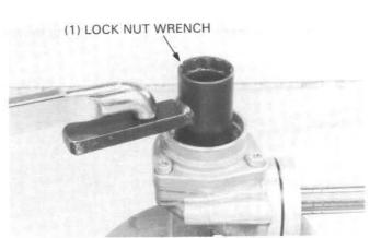
Hold the drive shaft with the shaft holder and tighten the inner race lock nut.
