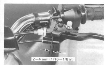
Adjust by loosening the lock nut and turning the adjusting nut.
