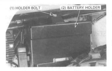
Disconnect the negative cable and then the positive cable and remove the battery.
