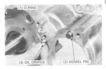
Install a new O-ring onto the output gear case.
