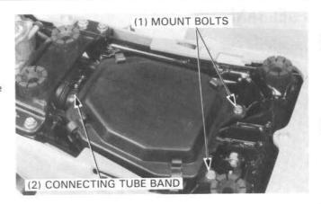
Loosen the air cleaner case-to-frame connecting tube band.
