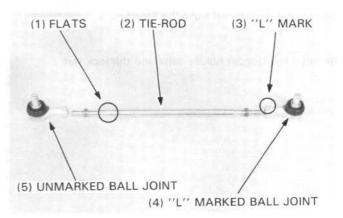
Thread the ball joints until the groove in the tie-rod threads enters the ball joint.
