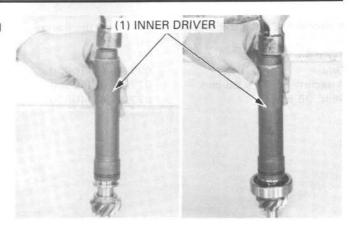
Place the pinion assembly into the gear housing and drive it into the gear case.
