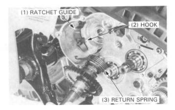
Install the kick starter assembly by turning it clockwise and aligning the ratchet with the ratchet guide.
