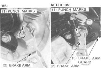
Connect the brake cables to the brake arm and install the adjusting nuts.
