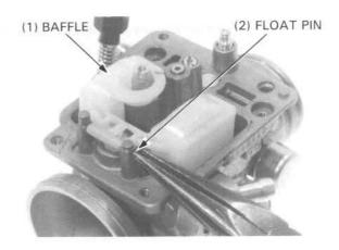
Inspect the float valve for grooves and nicks, and replace as required.
