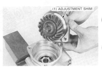
Backlash is changed by about 0.06 mm (0.002 in) when the thickness of the shim is changed by 0.10 mm (0.004 in).
