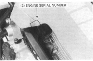
The engine serial number is stamped on the upper side of the right crankcase.
