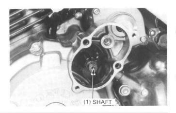
Install gear C, then install the gear A/B shaft and gear.
