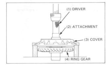
Remove the ring gear and adjustment spacer.
