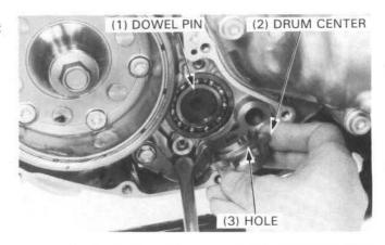
Tighten the drum center pin.
