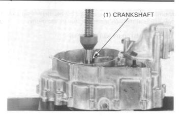
If the left crankshaft bearing remains on the crankshaft, remove it with bearing puller.
