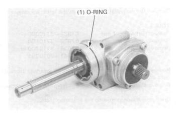
Install the output gear case onto the left crankcase and tighten the three mount bolts.
