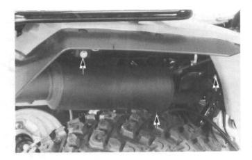
Install the exhaust pipe and muffler in the reverse order of removal.
