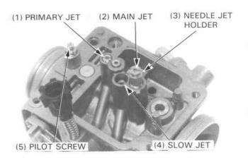
Inspect the pilot screw and each jet and replace them if they are worn or damaged.
