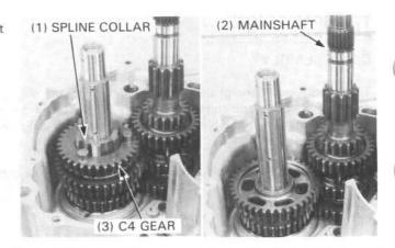
Remove the snap ring, spline washer, M4 gear and bushing from the mainshaft.
