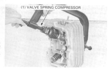
Tap the valve stems gently with a plastic hammer to firmly seat the cotters.
