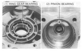
Drive a new pinion bearing into the case.
