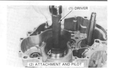
Align the timing marks on the balancer gear and crankshaft gear, and install the balancer and crankshaft into the left crankcase.
