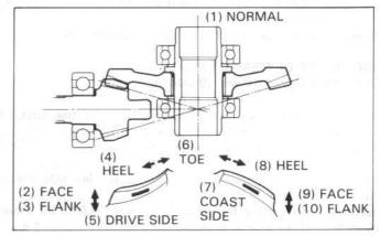
If the patterns are not correct, remove and replace the pinion spacer. Replace the pinion spacer with a thicker one if the contacts are too high, toward the face.
