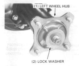
Install the axle nut and tighten to the specified torque.
