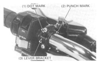
Install the master cylinder and front brake lever bracket with the "UP" mark on the holder facing up.
