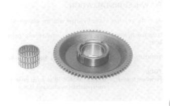
Check the rollers of the one-way starter clutch for wear or damage.
