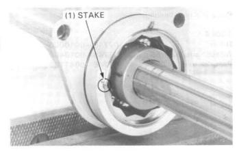
Remove the outer bearing race lock nut and lock washer. Discard the lock nut.
