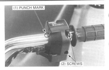
Install the rear brake lever bracket with the dot on the holder facing up. Align the end of the holder with the punch mark on the handlebar.
