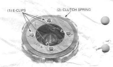
Check the weight springs for wear or damage, and replace if necessary.
