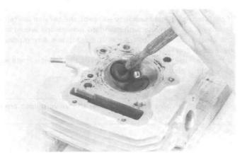
Inspect the width of each valve seat.
