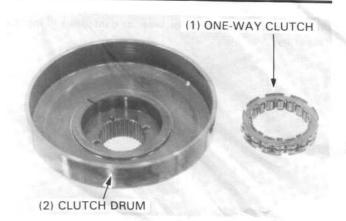
Install the one-way clutch into the clutch drum with its "OUT-SIDE" mark facing out.
