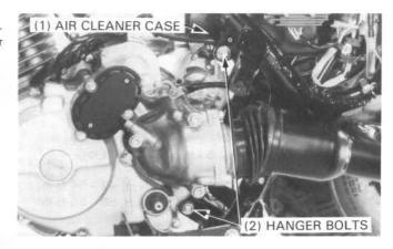
Remove the upper engine hanger plate bolts and plates.
