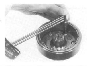
Install the starter driven gear into the one-way clutch by turning it clockwise.
