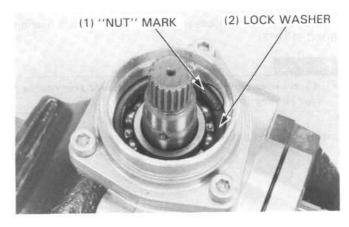
Install and tighten the driven gear bearing outer race lock nut.
