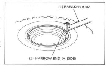
Insert the narrow end (A side) of the breaker arm between the tire and the rim.
