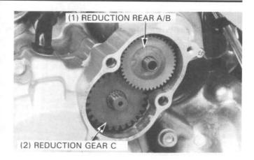
Install the gasket, dowel pins, and starter reduction gear cover with four bolts.
