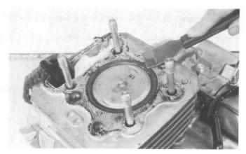
Place the bottom end of the cam chain guide into the groove in the right crankcase, and its bosses in the grooves in the cylinder upper surface.
