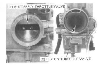
Make sure that the piston throttle valve is closed fully and there is no clearance between the throttle link and the piston throttle valve shaft arm.
