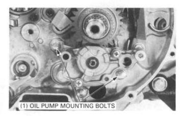
Remove the oil pump, primary drive gear and thrust washer. Remove the O-ring and two dowel pins.
