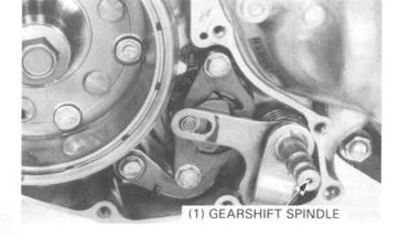
Remove the washer and return spring. Check the gearshift spindle for bend.
