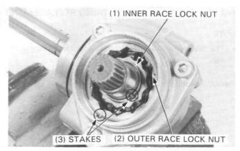
Remove the inner race lock nut and discard it.
