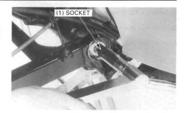
Tighten the lock nut while holding the right pivot bolt.
