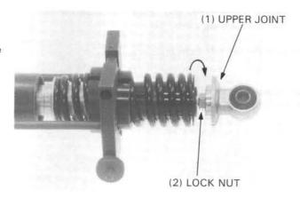
Inspect the spring for damage and measure its free length.
