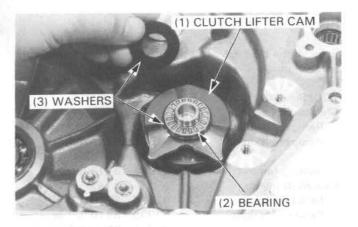
Install the lifter lever stay in the reverse order of removal.
