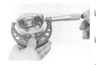
Measure the piston pin hole I.D.
