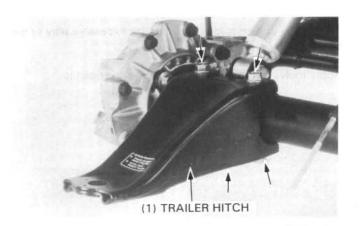
Disconnect the breather tube from the gear case.
