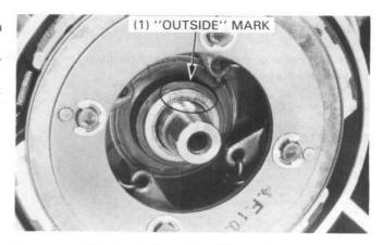
Apply a thread lock agent to the lock nut and tighten it. Hold the centrifugal clutch weight assembly with the clutch holder and tighten the lock nut by turning it counterclockwise.
