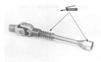
Set the universal joint in the compressor as shown and compress the spring.
