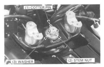
Remove the steering adjustment nut, top seal washer, dust seal, upper cone race and 28 upper steel balls.
