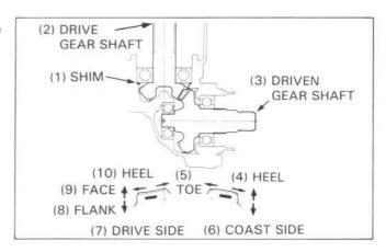
If the pattern is not correct, remove and replace the drive gear adjustment shim.
