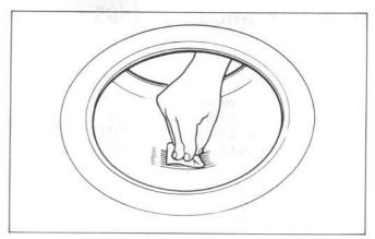
Apply cement over the area marked and allow it to dry. Remove the lining from the patch and center it over the injury. Press the patch against the injury using a special roller.
