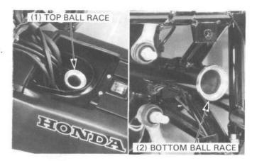
Drive in the new top and bottom ball races and reinstall the fuel tank.
