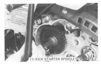
Remove the washer, collar, return spring, spring retainer, ratchet and ratchet spring.
