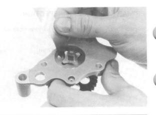
Remove the oil pump driven gear shaft from the oil pump cover and measure the pump end clearance.
