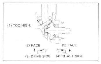
Replace the drive gear adjustment shim with a thicker one if the contact is too low.
