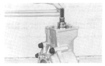
Stake the pinion bearing lock nut and install a new drive shaft bearing oil seal.
