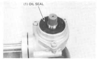
Unstake the driven gear bearing race lock nuts with a drill or grinder. Be careful that metal particles do not enter the bearing, and that the threads on the shaft are not damaged.
