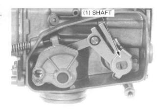
Remove the two screws attaching the valve arm to the valve and separate the valve and jet needle from the arm.
