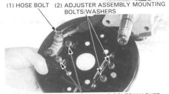
(3) WHEEL CYLINDER MOUNTING BOLTS/WASHER
