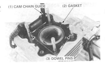
Install the cylinder head, and tighten the cylinder head cap nuts and socket bolts in the sequence shown in 2 or 3 steps.
