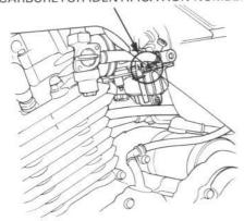
The carburetor identification number is on the carburetor body left side.
