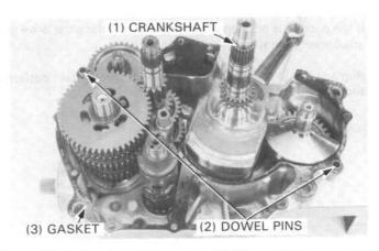
Tighten the left crankcase 6 mm bolts in a criss-cross pattern.
