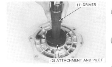
Install the ring gear shaft into the cover. It may be necessary to press the ring gear into the cover bearing.
