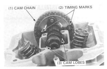
Tighten the cam sprocket bolt on the punch mark side first, then turn the crankshaft clockwise one turn and tighten the remaining sprocket bolt to the same torque.
