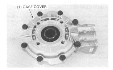
Place the cover in a press with the ring gear down. Make sure the cover is securely supported. Press the ring gear out of the cover.
