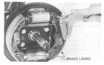
Remove the pins, pin holders, brake shoes and springs.
