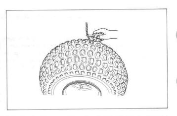
Inflate the tire and test the seal by dabbing a small amount of cement around the plug. Escaping air will cause a bubble in the cement. If there is leakage, remove the tire (page 13-3) and apply a cold patch to the inside of the tire as described. If a plug has been inserted, trim it even with the inner tire sur-
