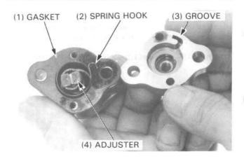
Screw in the adjuster all the way through the hole in the cover and install the tensioner lifter onto the cylinder. Tighten the two tensioner lifter mount bolts and release the adjuster.
