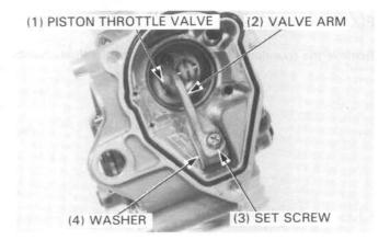
Pull the shaft out and remove the throttle valve and washer.
