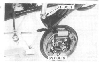
Bend up the tabs of the washer and remove the arm hinge bolt.
