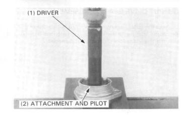
Press the output driven gear into the bearing.
