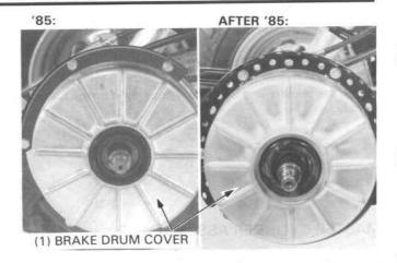
Loosen the rear brake cable adjusting nuts and remove the brake drum.
