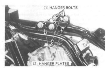
Remove the front hanger plate bolts and plates.
