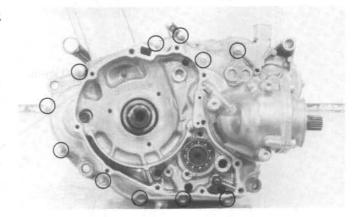
Tighten the right crankcase bolt to the same torque.
