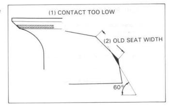
Refinish the seat to specifications, using a 45 degree finish cutter.
