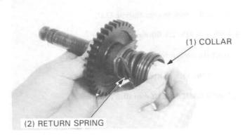
Hook the return spring onto the crankcase.
