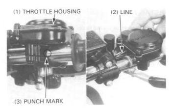
Install the handlebar upper holder cover and tighten it with the two bolts.
