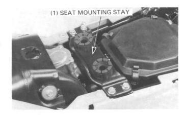
Loosen the air cleaner case connecting tube band.
