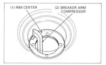
Keep the breaker arm horizontal and align the end of the compressor bolt with the arm hole.
