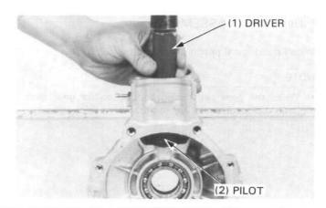
Drive a new ring gear bearing into the case.
