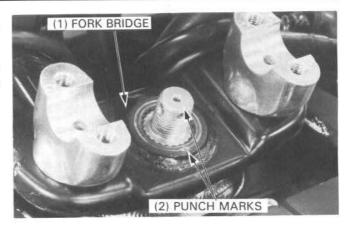
Install the washer and steering stem nut.
