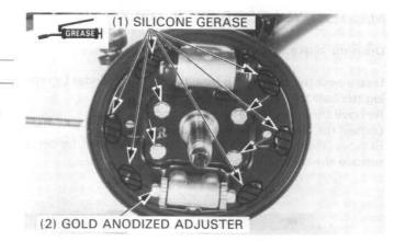
Install the brake shoes, springs, pins and pin holders.
