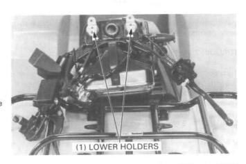
Install the lower holders onto the fork bridge and tighten the holder nuts.
