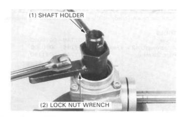
Remove the outer race lock nut and lock washer. Discard the outer race lock nut.
